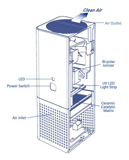
REME is an advanced oxidation technology utilizing UV light focused on a ceramic catalyst to produce light airborne hydro-peroxides capable of quickly reducing organic pollutants.
